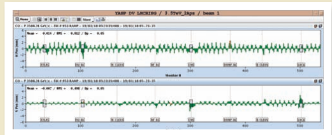
The difference between the orbit for beam 1 immediately after the first ramp to 3.5 TeV and the reference orbit for 450 GeV.
